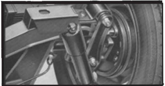
Each wheel of the Herald finds its own individual level. Coil springs controlled by telescopic direct-acting hydraulic dampers absorb all surface irregularities. There's an anti-roll bar, too, to ensure that the car (and you) stay on an even keel.
