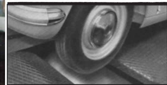
A Herald put through its paces. Special roller apparatus allows Triumph engineers to simulate varying braking speeds and road conditions. In this way the Herald's braking system is exhaustively tested before the Herald even goes on the road.
