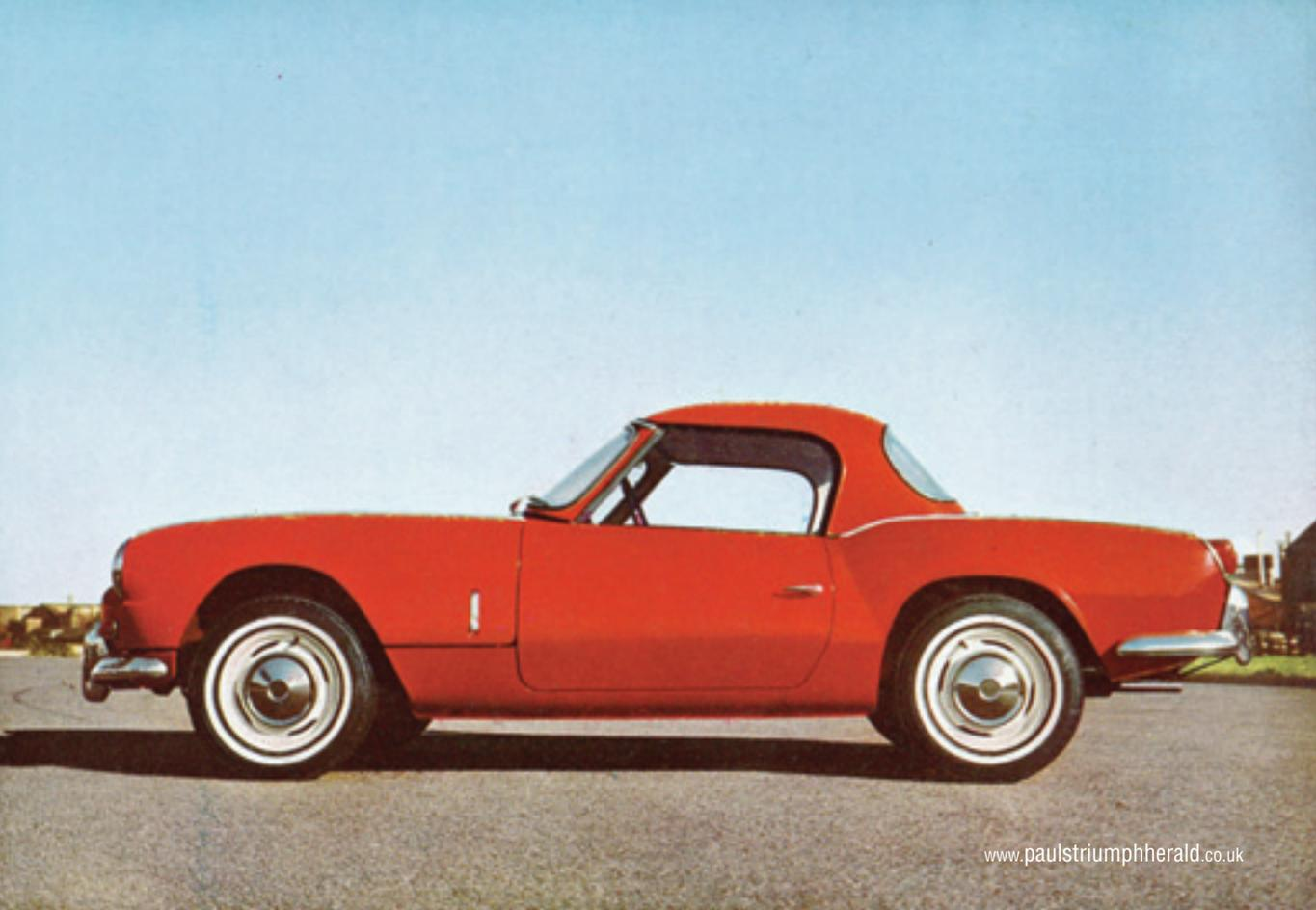
**A detachable steel hard top now adds a snug, sleek Coupé to the exciting Spitfire range. It can be fitted or removed in minutes. Just six bolts are employed (two of which locate through the hood stick sockets for soft top use) so that adding or detaching the hard top is an easy, speedy one-man operation.**
